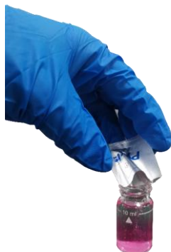
Figure 12. Add DPD powder to sample.
