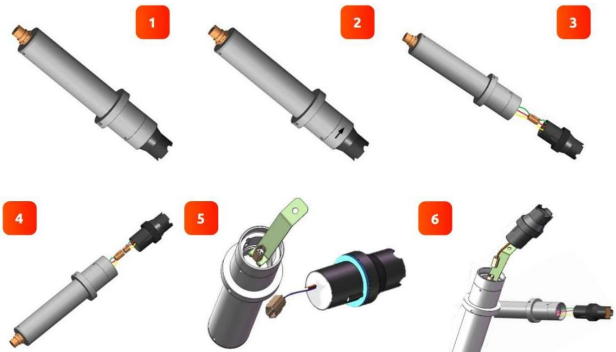
Figure. 61 - Replacing EH-765 pH, ORP and Sulfite Electrode Head
