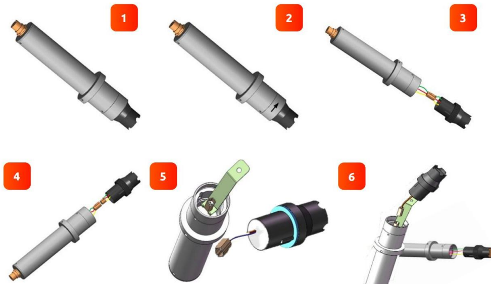
Figure. 58 - Replacing EH-765-01 pH and Oxidizer Electrode Head
