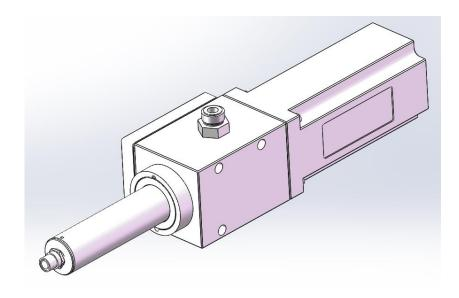
Step 7. Reinstall the sensor retaining nut to the position shown in the picture.
