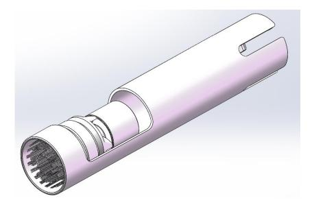
**Step 5.** Fit the new brush in the tapered end position of the tool as shown in the picture and insert it into the hole, gently press on the tool until the brush has been adequately installed onto the drive shaft of the brush motor within the flow assembly, then remove the tool. Your brush has been replaced.
