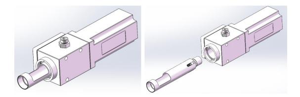
**Step 4.** Remove the brush when it reaches the tool grooved opening.
