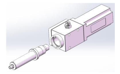
**Step 3.** Insert the extraction tool with the slotted end first until the head of the tool snaps onto the collar of the brush.
