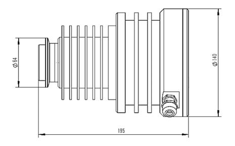
Tri-Clamp Flow Assembly Dimensions (mm)
