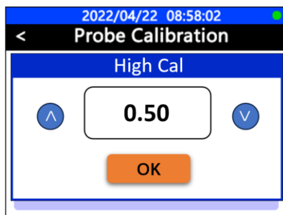
Figure 15. High (slope) Calibration
