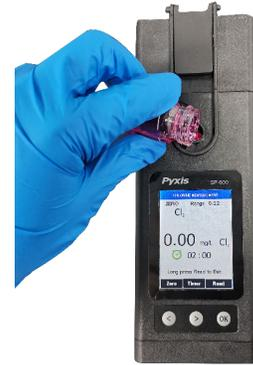
**Figure 19.** Fill sample cell with developed sample
